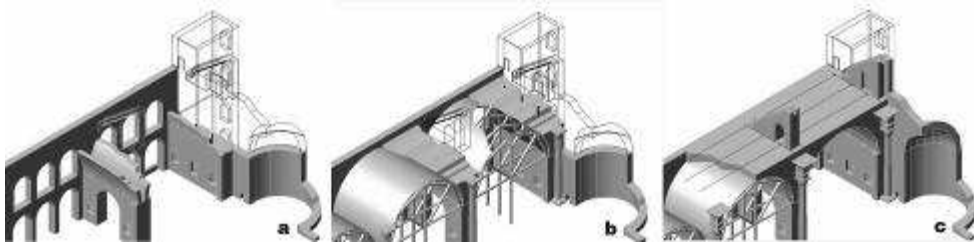
Figure 11 Reconstruction of the building sequence of the south-west aisle. a) arrangement of the terracotta tubes at the spring of the two concentric rings of lattice ribbing forming the shell of the barrel vault, in connection with the lodging of the main beams of the centering, marking the correct positioning of the buttressing arch; b) lay out of the vault conglomerate, in parallel layers up to the upper end of the tubes; c) removal of the centering, check of the thickness of the concrete and of the vertical line of the tubes, using them to fix the exact position of the buttressing arches. The floor of the terrace will eventually hide the tubes.
