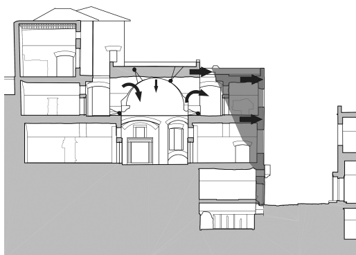
Figure 5. The Southern building weak behaviour and the collapse mechanism in case of transversal seismic action.
