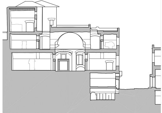
Figure 4. The Great room, in the centre, which divides the Northern building, on the left, from the Southern one, on the right; note the lower level of via Biberatica respect the Hall.
